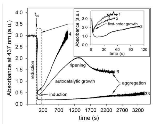
FIG. 7: Evolution of the absorption for reactions with different concentration of NaOH as a function of time at room temperature,  $[\text{Pd}]_0 = 10\text{mM}$ ,  $V_{\text{total}} = 5\text{ ml}$ .
