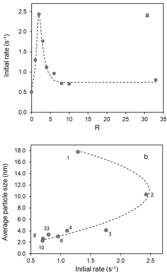
FIG. 9: (a) Initial rate for different R ratios. (b) Particle size function of the initial rate, (R value is indicated).
