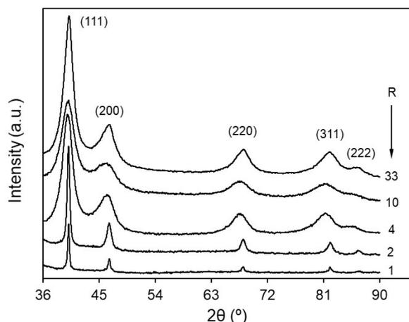
FIG. 3: XRD patterns of Pd nanoparticles for different R, as indicated.
