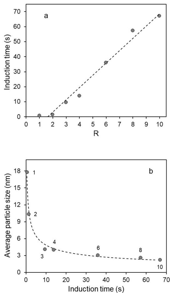
FIG. 10: (a) Induction time for different R ratios. (b) Particle size function of the induction time, (R is indicated).
