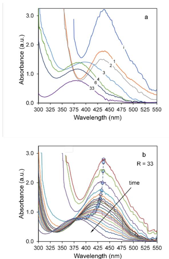
FIG. 12: (a) Variation of the characteristic Pd absorption bands for different  $R$  when the induction time is equal to zero. (b) Maximum absorbance peak evolution for  $R = 33$ .
