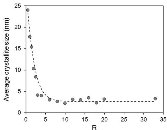
FIG. 5: Average size of Pd nanoparticles from XRD analysis.
