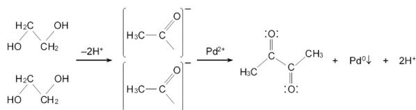
FIG. 1: Reduction reaction of metallic ions by ethylene glycol oxidation.
