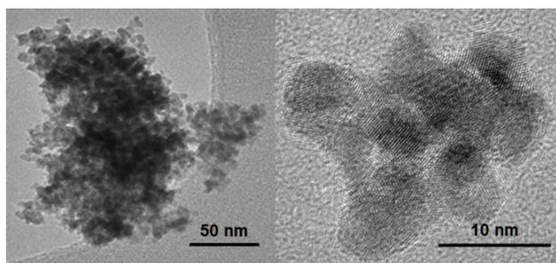
FIG. 4: TEM image of Pd nanoparticle aggregates obtained for  $R = 10$ .
