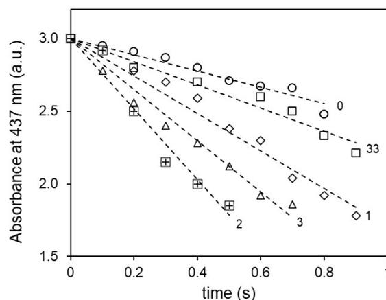
FIG. 8: Absorbance ( $\lambda = 437\text{ nm}$ ) vs. time of the initial region of the  $\text{Pd}^{2+}$  reduction curves at different R.
