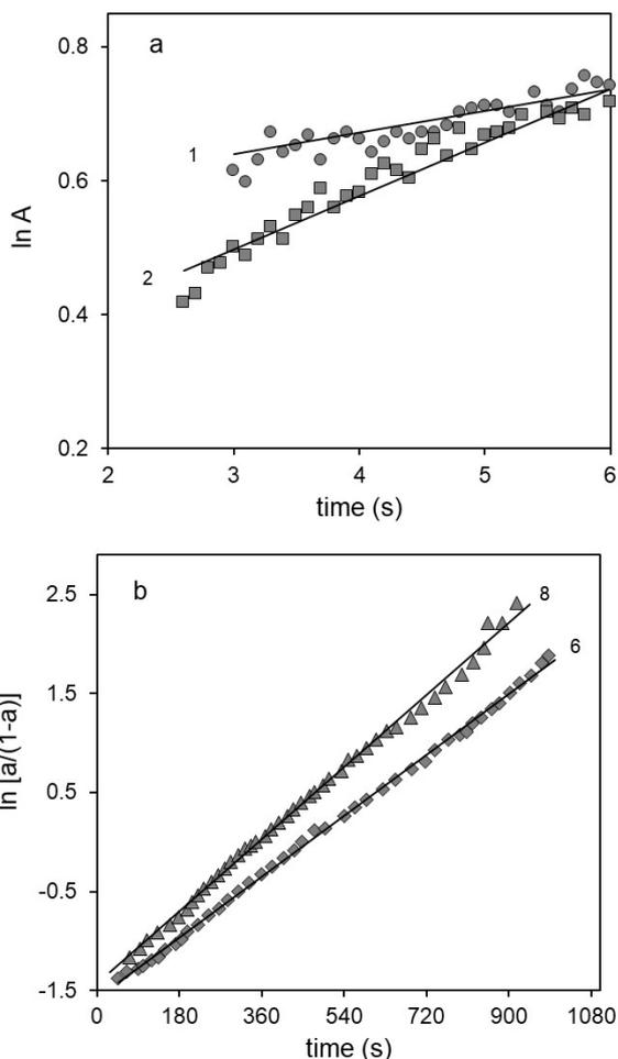
FIG. 11: (a) Absorbance as a function of reaction time (first-order growth). (b) Plots of  $\ln[a/(1-a)]$  as a function of reaction time (autocatalytic growth).
