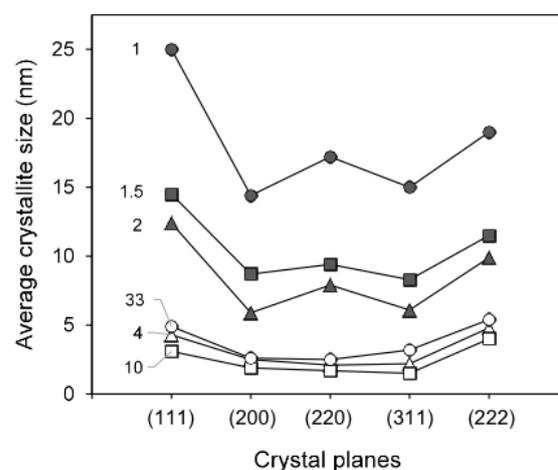
FIG. 6: Average crystallite size of Pd nanoparticles for different R obtained from XRD analysis by applying the Scherrer equation.
